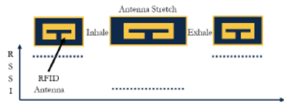
Fig. 3: Respiration rate monitoring from RFID data by correlating the change in received signal strength to antenna size modulation due to respiratory activity
