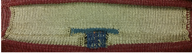
Fig. 2. Knit Bellyband Antenna with a folded dipole antenna shape. Silver part of the antenna is knitted using conductive yarns.
