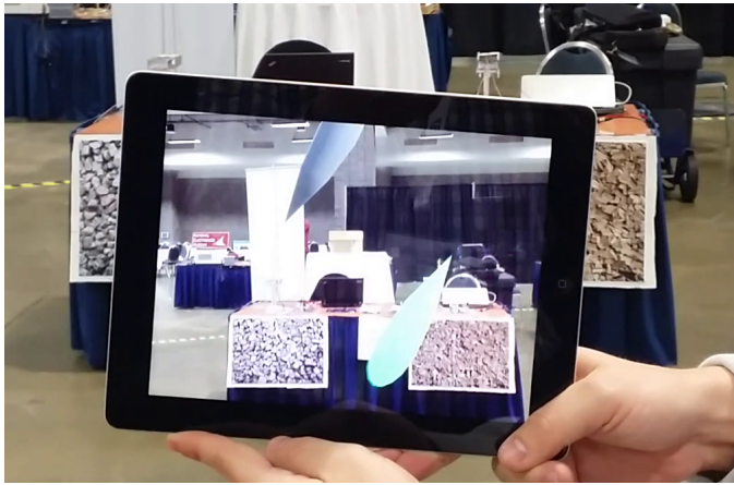
Fig. 2: BeamViewer mobile frontend. The blue and green antenna beams are annotated by the AR toolkit and correspond to pre-measured antenna radiation patterns.
