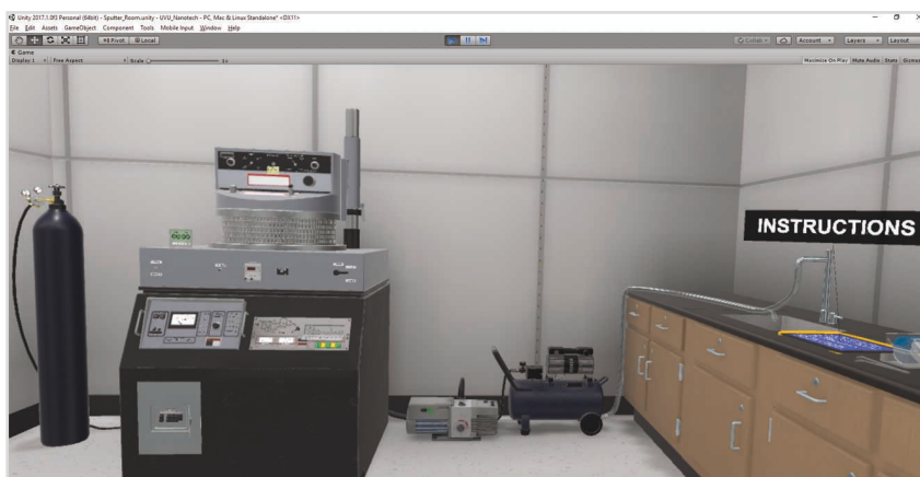
FIGURE 10 A VR view of the sputtering room. From left to right: the argon tank, a PerkinElmer 2400 RF sputtering unit, the roughing pump, and the air compressor.
