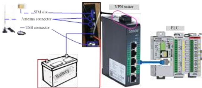
Fig. 4. Schematic of connection between VPN, PLC, and power
