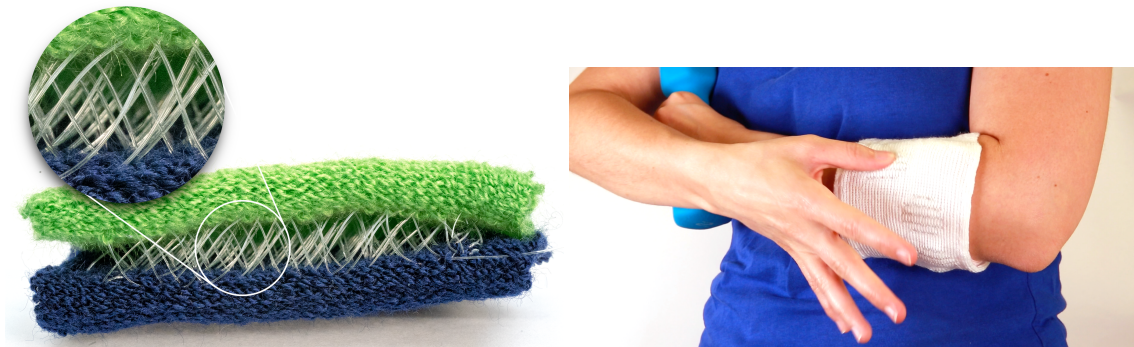
Fig. 1. Weft knit spacer fabric (left) can be used as a material in user interface design, by, e.g., by integrating dimensional soft capacitive buttons into a knit surface (right).
