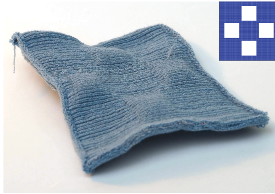
Fig. 7. Differences in tuck spacing can be used to generate fabrics with areas of different thickness.
