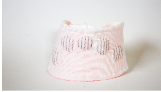
Fig. 15. The soft control pad from Figure 1. Different thickness provide tactile cues to the location of capacitive button traces.
