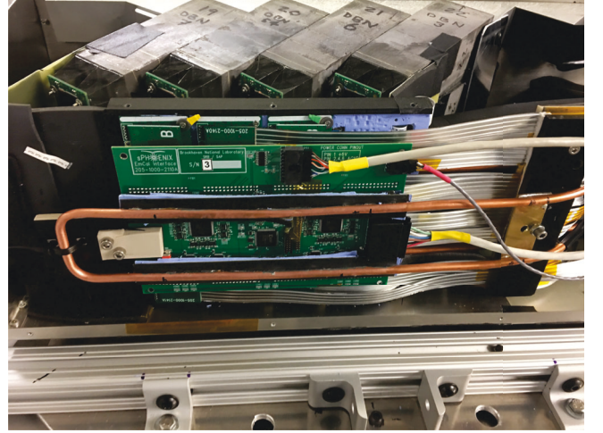
Fig. 4. EMCAL prototype showing the EMCAL blocks, light guides, SiPMs, electronics and part of the cooling system.
