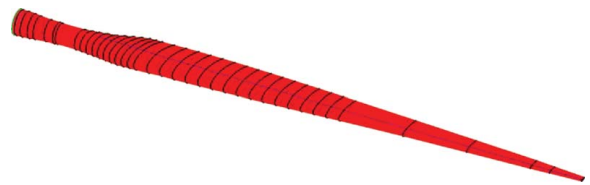
Fig. 9 CX-100 blade model created in NUMAD for ANSYS input file generation and finite-element analysis
