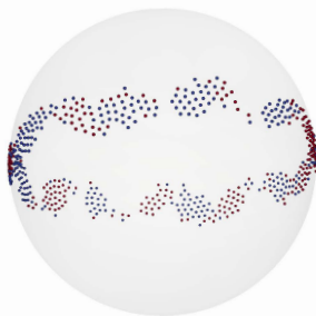
Figure 5. Particle distribution at t = t_f for N = 512 particles with E_0 = 400\text{V/mm} .
