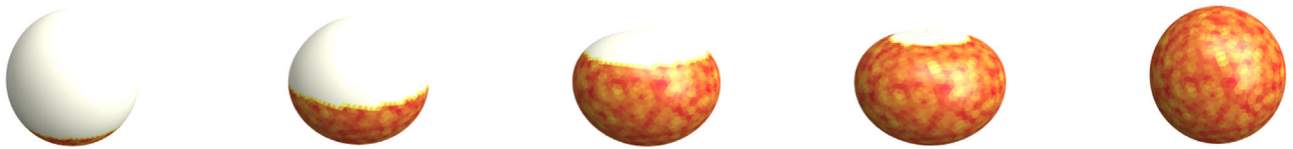
FIG. 4. Low-energy shapes of NPs with Janus patches of charge density \sigma = 0.06 \text{ e/nm}^2 and elastic moduli \kappa_b = 3 and \kappa_s = 75 (in units of k_B T ). Patch size increases from left to right as p = 0.25, 0.50, 0.75, 0.90, 1.0 ; other parameters are the same as in Fig. 1. Anisotropy of the surface charge itself causes deformation; when uniformly charged ( p = 1 ), the NP does not deform.
