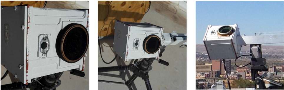
Fig. 2. Germanium and neutral density lenses are attached to the IR and VI cameras, respectively, to filter the light beams and protect the cameras from weather hazards (left). The solar tracker's servomotors are mounted on the tripod and screwed to a metallic structure which counterbalances the enclosure's weight (middle). The sky-imaging system (right) installed on the roof of a UNM building.
