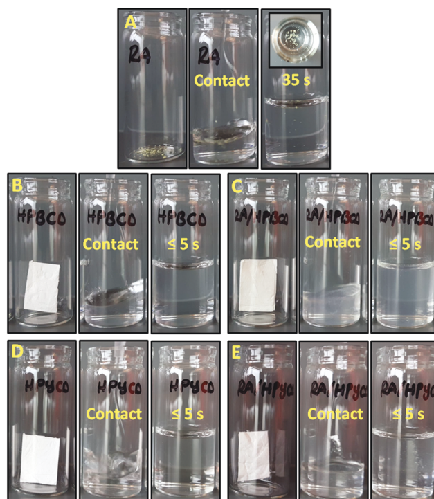
Fig. 7 The dissolution behavior of samples in water. (A) Vitamin-A acetate powder, (B) HPβCD-NW, (C) Vitamin-A acetate/HPβCD-NW, (D) HPγCD-NW and (E) Vitamin-A acetate/HPγCD-NW. These images were captured from Video S1.†
