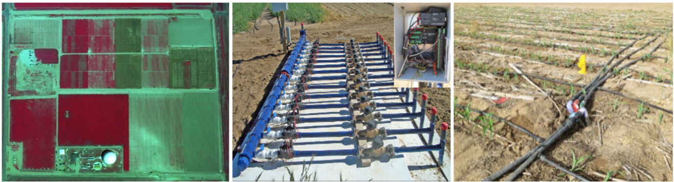
Fig. 1. Aerial view of 16 Hectare of Greeley, Colorado, USDA experimental site (left); Irrigation control, monitoring system and turbine flow meters (middle); Drip irrigation pipes in field (right). Taken from (Trout, 2016).
