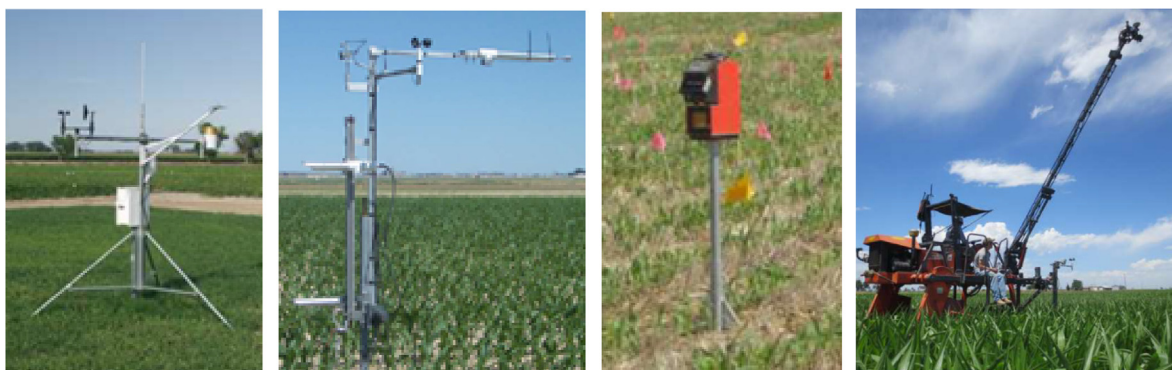
Fig. 2. (a) Weather Station, (b) Bowen Ratio Energy Balance meter, (c) Neutron Moisture Meter, and (d) High clearance reflectance tractor taking canopy ground cover image. Taken from (Trout, 2016).
