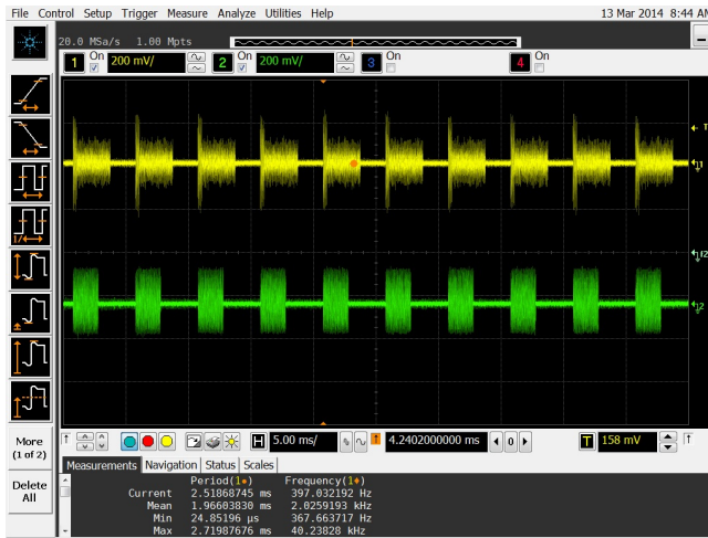
Figure 12: Reactive jamming of WiMAX downlink packets from an Airspan Air4G base station.
