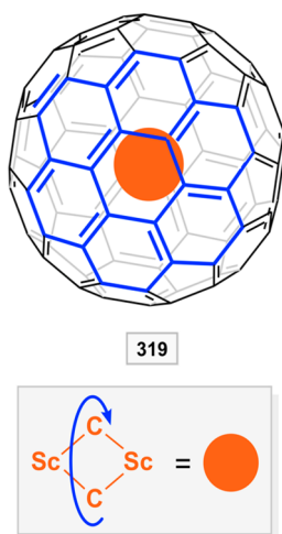
Figure 68. Solid endohedral fullerene C_2Sc_2@C_{84} (319), considered an example of a quantum gyroscope.
