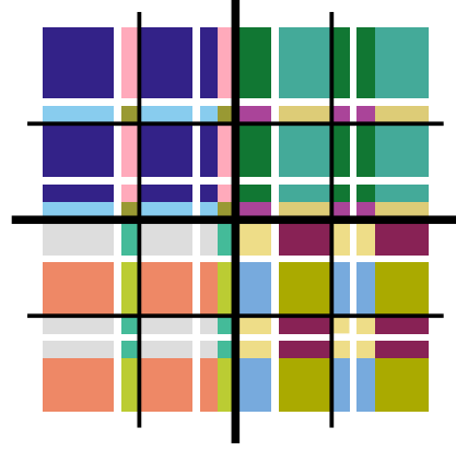
Fig. 4: Subtiles gathered for computing a layer of an RBT for butterflies of size n/2 . All submatrices of the same color are gathered onto the process owning the upper left entry of the color for the computation.
