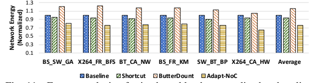
Fig. 11. Energy analysis of mixed workloads, normalized to baseline.
