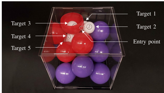
Fig. 19. Experimental setup for the preliminary user study. The targets to reach are small white plastic spheres, numbered from 1 to 5. The environment is created using larger plastic spheres, with violet ones representing areas far from the targets and red ones representing potential obstacles.
