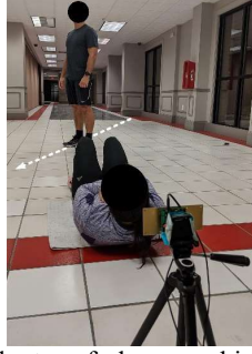
Fig. 4. Experimental setup of a human subject doing sit-ups while another person walking by.
