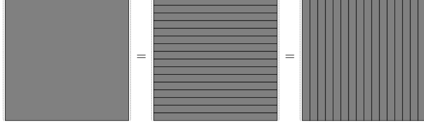
Figure 8: The left figure is a complementary two-dimensional low-rank kernel matrix K . Assume that the depth of the quadtrees of column and row spaces is 3. The middle figure illustrates the root-leaf partitioning that divides the row index set into 16 subsets as 16 leaves. The right one is for the leaf-root partitioning that divides the column index set into 16 subsets as 16 leaves.
