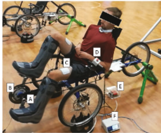
Fig. 12. Participant 4 seated on the motorized recumbent FES cycle. Label A indicates the encoder, label B indicates the powermeter, label C indicates the electrodes, label D indicates the emergency-stop, label E indicates the filter card, and label F indicates the stimulator. The electric motor is coupled to the drive chain below the seat.
