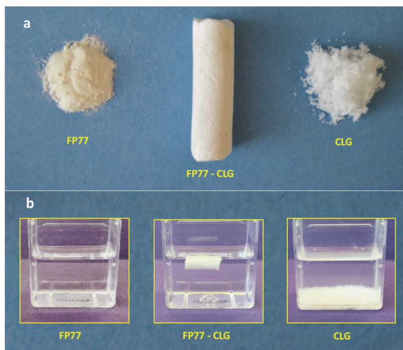
Fig. 5 (a) Images of FP77, CLG and the resulting composite material – FP77-CLG as solids and (b) after dissolution or immersion in aqueous solution
