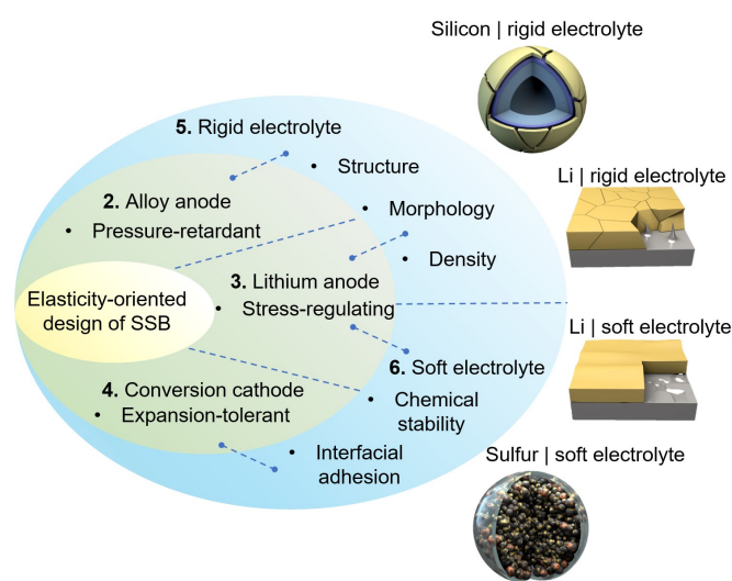
Fig. 2 Design strategies for the solid-state high-strain electrodes.
