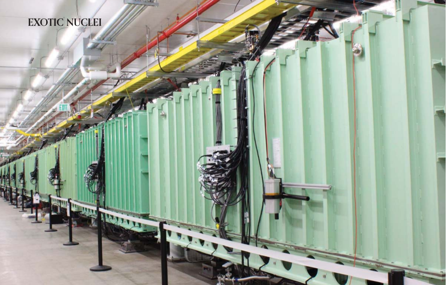
FIGURE 4. THE FACILITY for Rare Isotope Beams is taking shape as the highest-energy superconducting heavy-ion linear accelerator in the world. When it begins operating in 2022, the facility will be able to accelerate all ions from hydrogen to uranium to at least 200 MeV/nucleon and produce thousands of rare isotopes by in-beam fragmentation. (Courtesy of the Facility for Rare Isotope Beams.)
