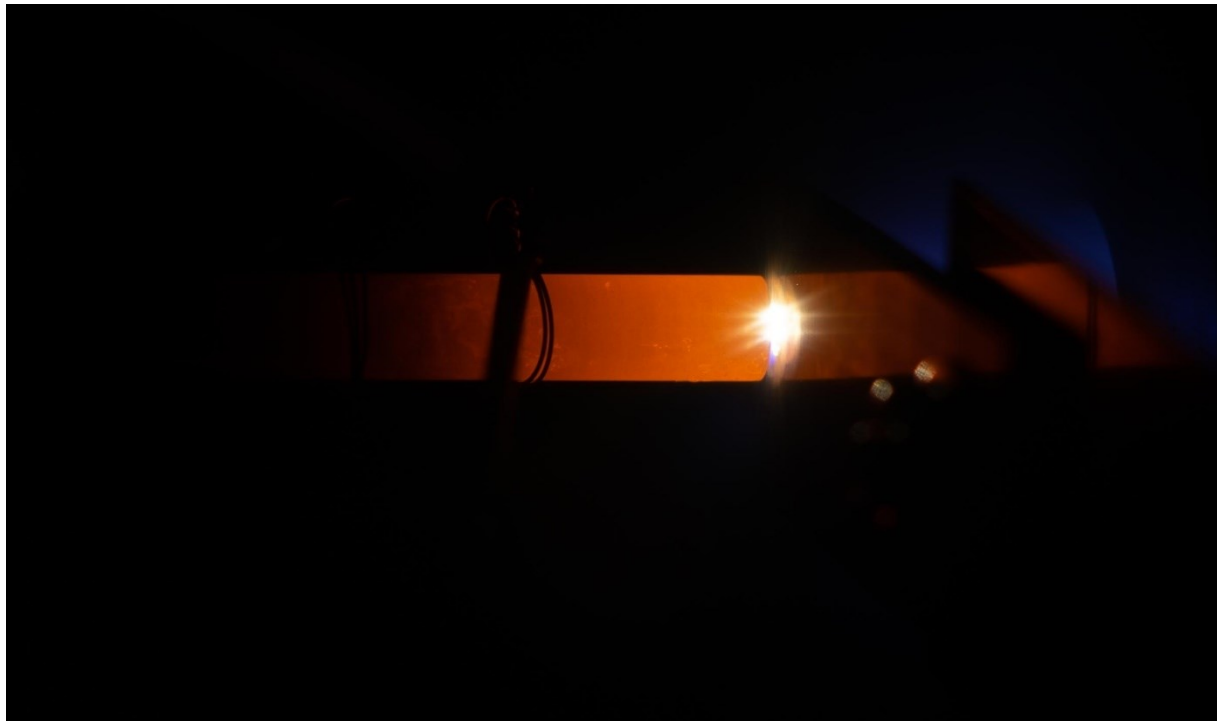
Figure 6: The hollow cathode being fired with an anode current of 1 A.-Note that the dark streak on the right is the thermocouple and Nickel-Chromium wires securing the thermocouples to the cathode.
