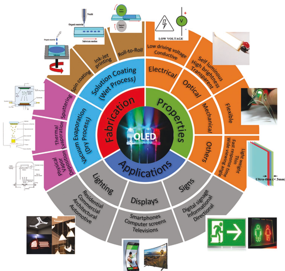
Figure 1. Schematic illustration of organic light emitting diode (OLED) from three aspects: fabrication, properties, and applications.
