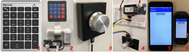
Figure 5: Six devices are used in our experiments, including two keypads (a plastic keypad labeled as 1, and a rubber one as 2; in either case, we only use one button for pairing); two knobs (a large knob labeled as 3, and a small one as 4); two touchscreens (a 5.2" Google Nexus 5X labeled as 5, and a 2.45" Unihertz Atom labeled as 6).
