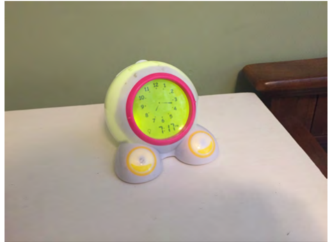
Figure 4: A child-friendly clock which glows green when the child is allowed to come to their parents’ room, and red when it’s too early.
