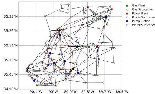
Fig. 3.: The topology of the gas-power-water system in Shelby County, Tennessee.
