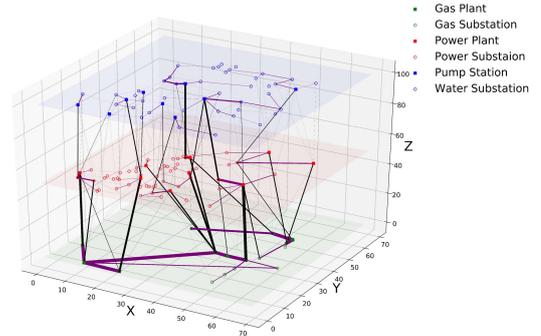
Fig. 4.: The gas-power-water system of Shelby County. The nodes in green, red, and blue represent facilities in gas, power and water networks. Intra-network flow is in purple while inter-network flow is in black. The thickness of each link represents the capacity of flow.
