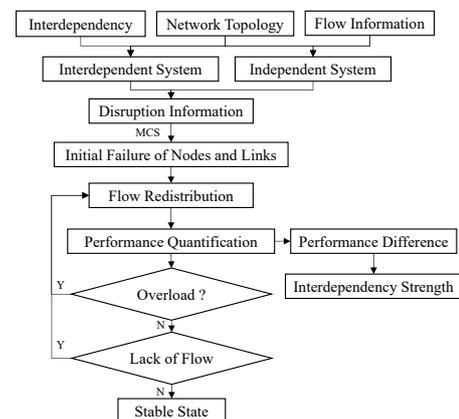
Fig. 1.: Framework for quantifying interdependency strength of infrastructure systems.
