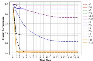
Fig. 5.: The performance deterioration of the system under different seismic intensities.
