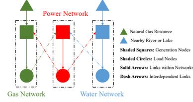
Fig. 2.: An interdependent gas-power-water system.
