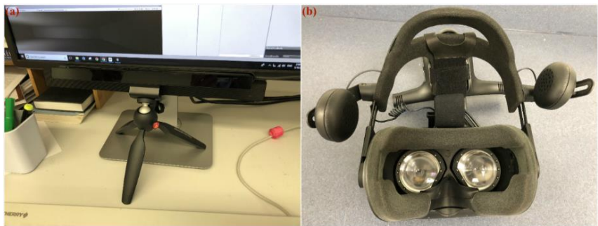
Figure 2. The Eye trackers used in this study (a) Tobii Pro X3-120 eye tracker; (b) Tobii Pro VR Integration eye tracker
