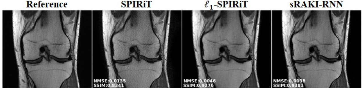
Fig. 2: A proton-density knee dataset from the NYU FastMRI database, retrospectively undersampled using a random variable density pattern at rate 4, and reconstructed using SPIRiT, \ell_1 -SPIRiT and sRAKI-RNN. sRAKI-RNN yields the best performance in terms of reconstruction noise, reduction of blurring artifacts and quantitative metrics.
