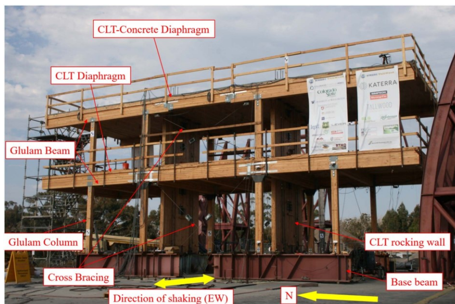
Fig. 1. Two-story CLT rocking wall structure.
