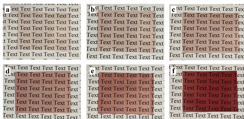
Figure 3. (a–f) Photographs of composite films (PMMA-54) filled with P-54 at different particle weight loadings: (a) 0.25 wt %, (b) 0.5 wt %, (c) 0.75 wt %, (d) 1 wt %, (e) 2 wt %, and (f) 4 wt %.
