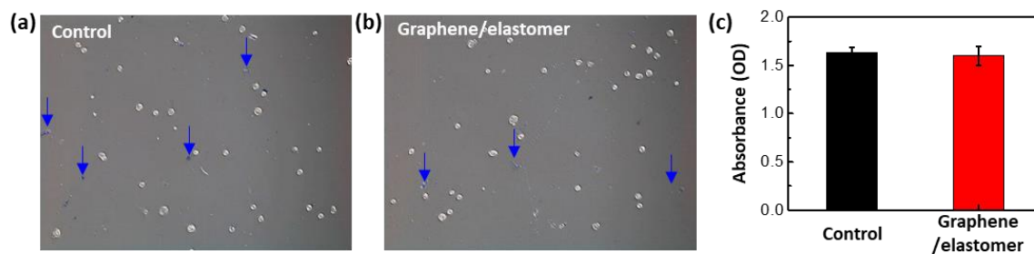
Figure S4. Biocompatibility of printed electrodes. (a,b) Optical microscopic images of cultured keratinocyte cells after exposure to original DMEM (a; control sample) and DMEM with graphene/elastomer (b) after 7 days of culture. In the images, small blue dots represent dead cells (pinpointed by blue arrows). (c) Comparison of cell absorbance of the control and graphene electrode.
