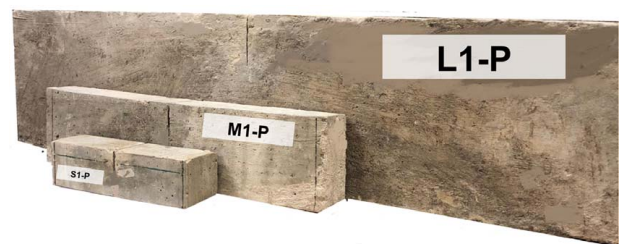
Fig. 2 Concrete test specimens scaled geometrically in two dimensions
