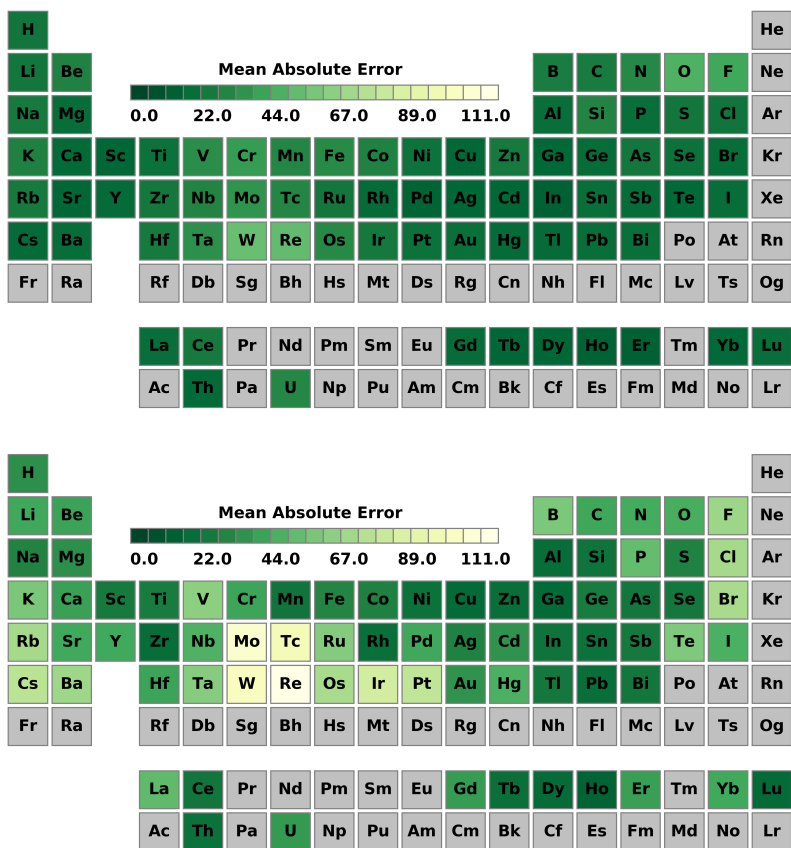
Fig. 4 Mean Absolute Error of bulk modulus predictions using Oliyntyk (Top) and Random (Bottom) when compounds that include the shaded element are heldout during training and then tested on.
