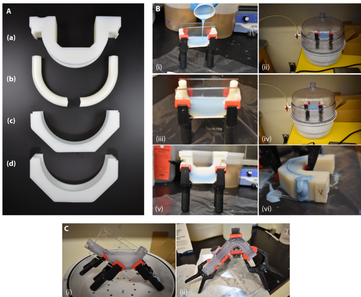
Fig. S5 Silicone casting methods. (A) 3D-printed multi-component mold for fabricating actuators with an initial bend angle of 180^\circ . The mold is made up of: (a) a mold with inlaid grooves for fibers for the inner half of the actuator, (b) inner cores, (c) component to align the inner cores, and (d) a mold with inlaid grooves for fibers for the outer half of the actuator. (B) The silicone casting process depicting: (i) pouring, (ii) 1 st degassing step, (iii) introduction of the inner cores, (iv) 2 nd degassing step, (v) bringing the mold halves together, and (vi) clamping the mold for curing. (C) Analogous casting process for the multi-segment actuators to replicate diaphragm motion. (i) The concave piece is used to degas the silicone. (ii) The molds for casting the first layer require more points of clamping.
