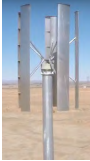
Figure 2: Photographs (left) and specifications (right) of the helical-bladed UGE turbine (top) and the straight-bladed WPE turbine (bottom). The blade twist of the UGE turbine is \tau = 0.694 \text{ rad} \cdot \text{m}^{-1} .
