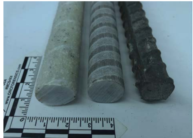
Fig. 1. Bar types. From the left: GFRP Type-A, GFRP Type-B and steel Type-S.
