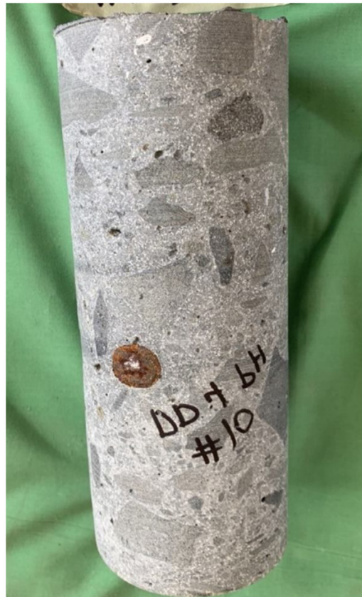
Fig. 2. Corroded steel reinforcement in an extracted cored specimen (Core #10 – Region II). The steel rebar is likely from the repairs done in the 1990s.
