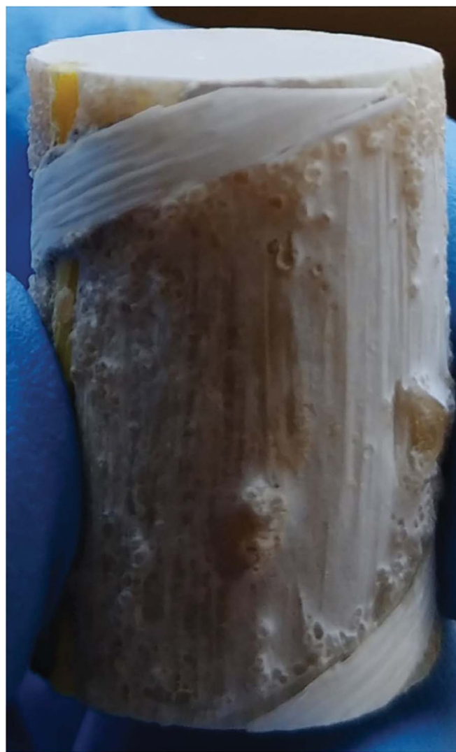
Fig. 3. Part of the helical wrap fell off one bar from the Cuyahoga Bridge during 50°C water absorption testing.
