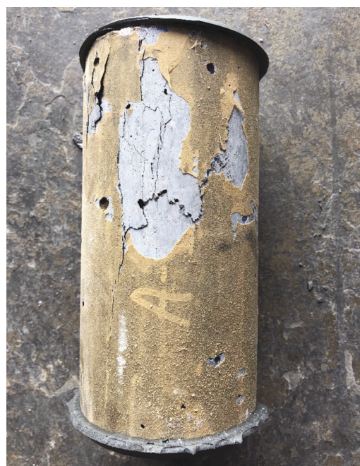
Fig. 7—Layer of leached material covering surface of concrete cylinder cast with reference concrete (Mix A) after immersion in seawater at 60°C (140°F) for 24 months.
