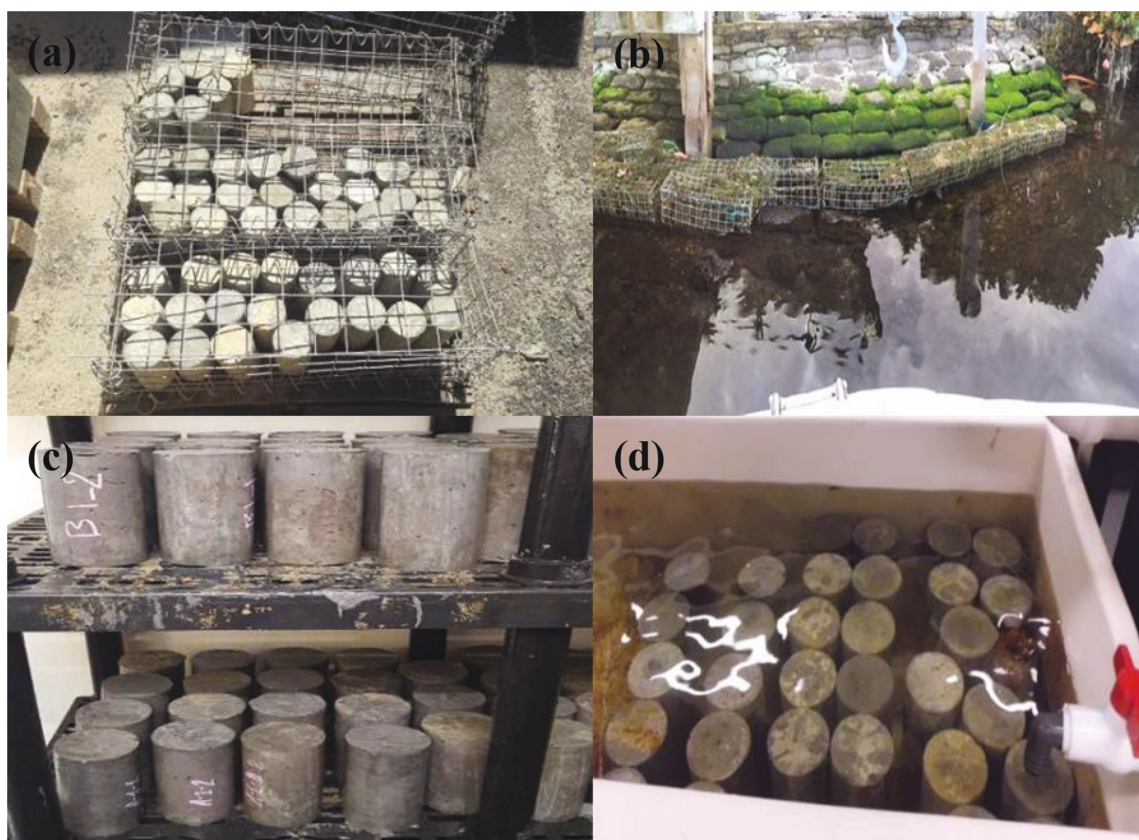
Fig. 1—Different curing regimes: (a) subtropical environment; (b) tidal zone; (c) moist curing; and (d) immersed in seawater at 60°C (140°F).
