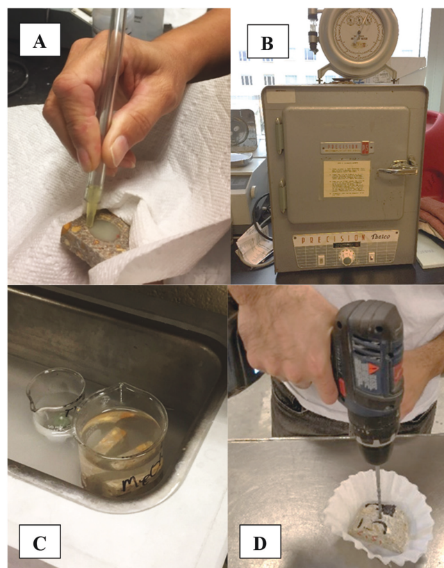
Fig. 7—Preparations of specimens: (a) air drying; (b) oven drying; (c) sonic bath; and (d) drilling to get concrete powder.
