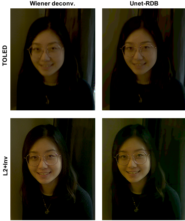
Fig. 14. Comparison of deblurring methods. We compare Wiener deconvolution and UNet-RDB on a selfie captured under conventional T-OLED and our optimized display. We use display masks of 150 DPI.
