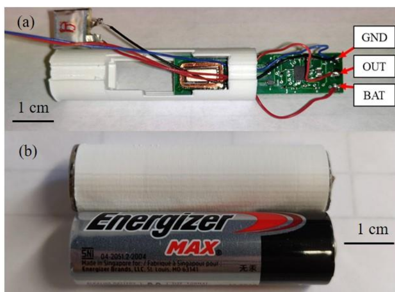
Figure 7. (a) Orientation of the PMC/EWPT receiver subassembly and pad labels, and (b) completed AA-sized prototype next to a commercially available Alkaline AA battery.
