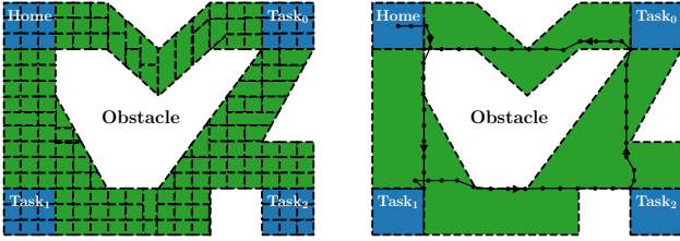
Fig. 3. The abstractions in Example 3 using bisimulation (left) and divergent stutter bisimulation (right). A path using the synthesised controller is shown for the divergent stutter bisimulation.
