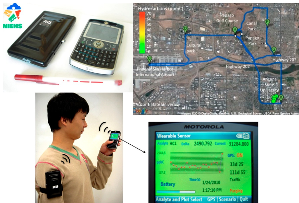
Figure 14. A wireless wearable chemical sensor based on tuning fork sensors for selective and real-time detection of hydrocarbons (traffic pollutants) and acid vapors with sensitivity of ppb–ppm range, spatial resolution and signal processing based on a cell phone app. The device was used to monitor the exposure of individuals to traffic pollutants.
