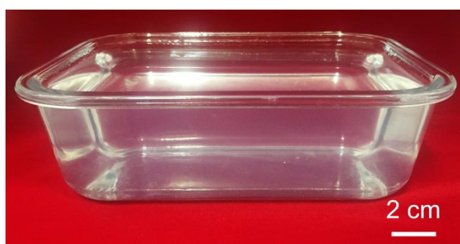
Figure S2 The bath is low-cost (<$2/lit), easy and fast to prepare in large quantities, and it is transparent, which facilitates process monitoring.
