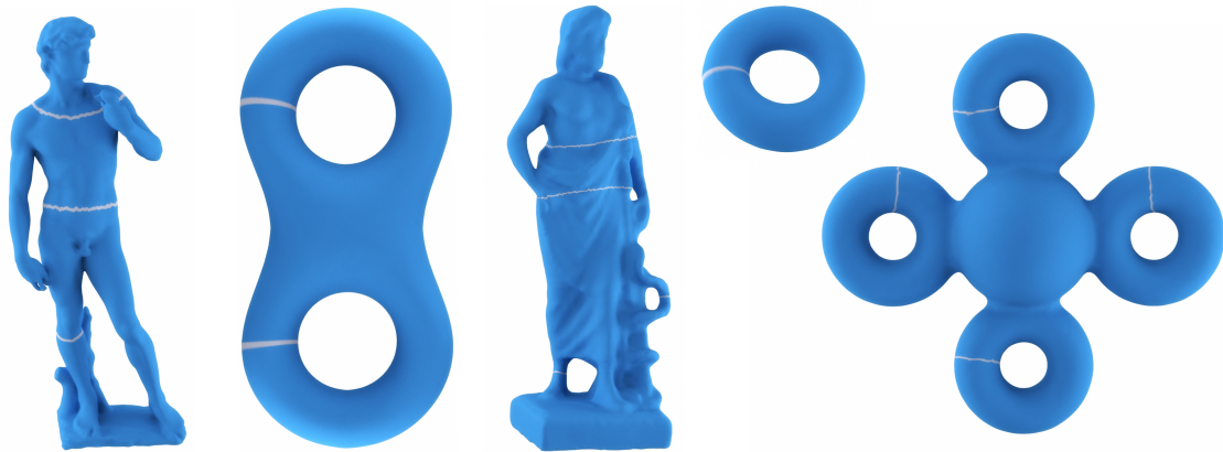
Figure 21. Examples of cut system curves on triangulated surfaces.
