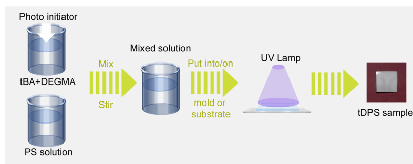
Figure 1. Schematic showing processing steps to prepare a tDPS composite.
